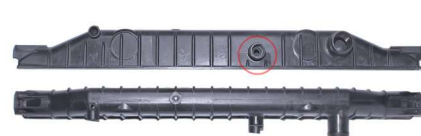
665 / S10 2013> Diesel Inferior Manual P/ Sensor no Meio
